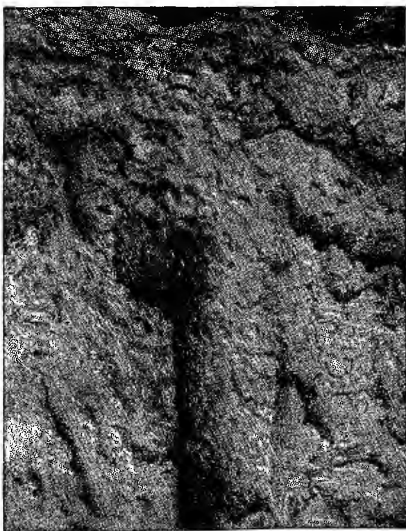
FIG. 75.—FRACTURE OF MASSIVE IRON.
